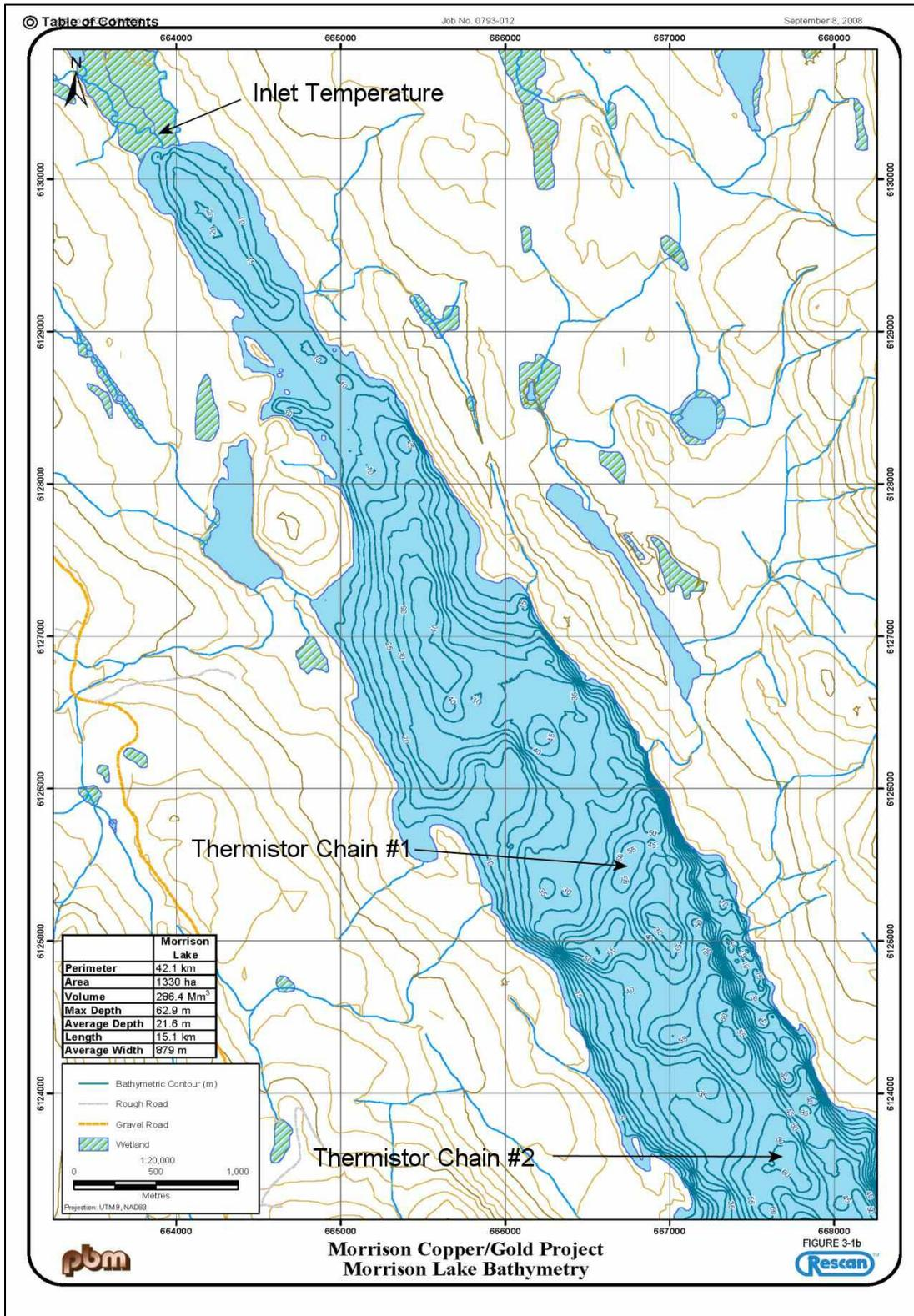
Figure 2 Bathymetric map with temperature monitoring stations on northern basin.
