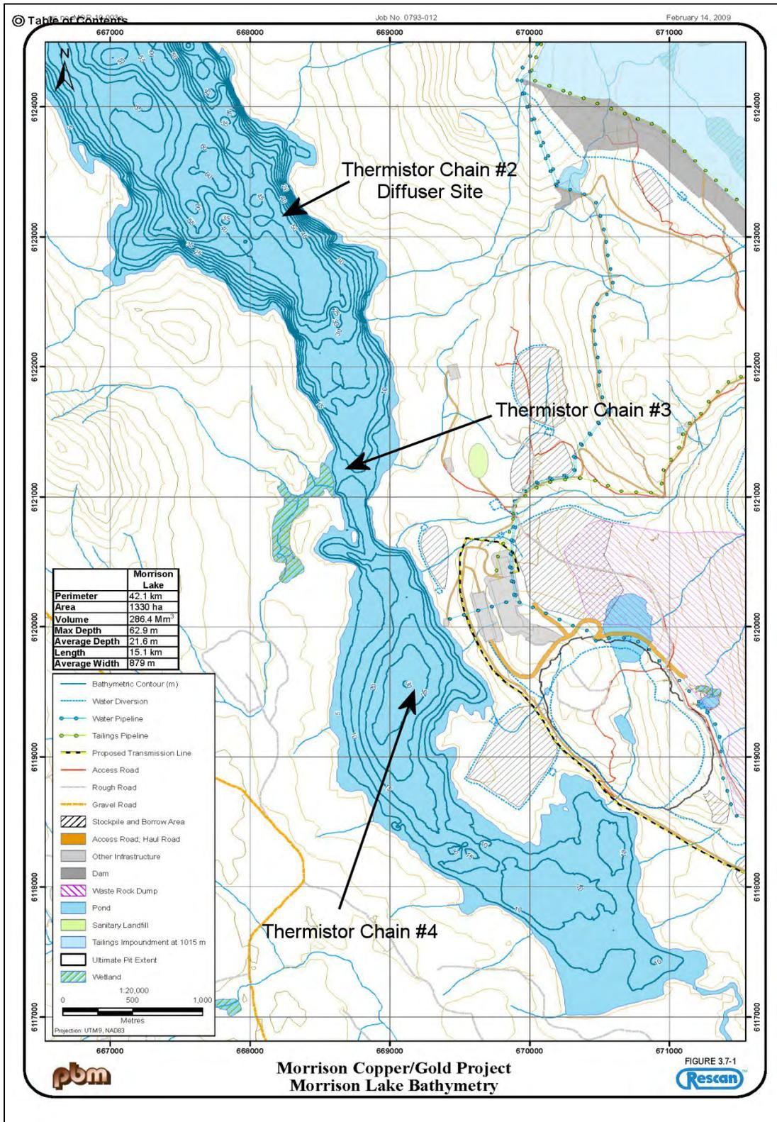
Figure 3 Bathymetric map and temperature monitoring stations on southern basin.
