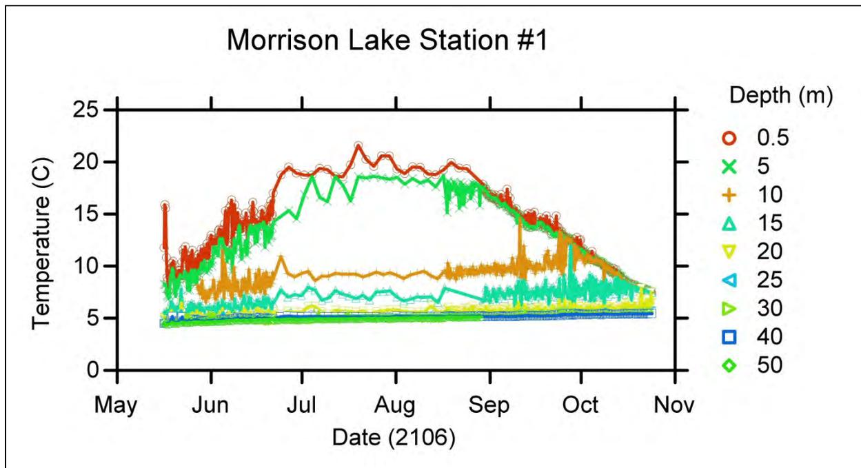
**Figure 10 Temperature data from Station #1 thermistor chain.**
