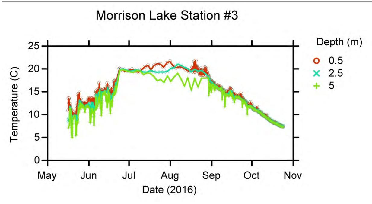
Figure 12 Temperature data from Station #3 thermistor chain.
